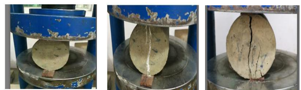
Fig -3: The split tensile test proceedings before and after test testing
