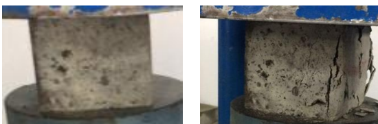
Fig -1: Compressive strength test before and after testing
