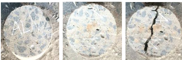
Fig -4: Impact test proceedings of the specimen before testing, initial crack and failure
