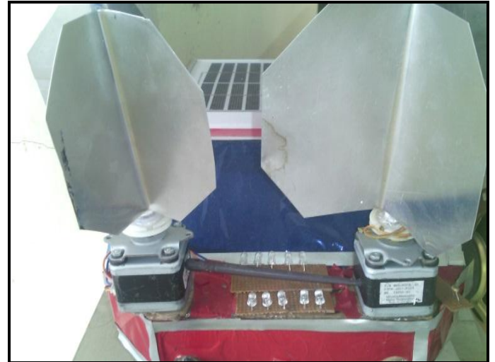
Fig -3: Propeller and dynamo for charging battery using wind energy
