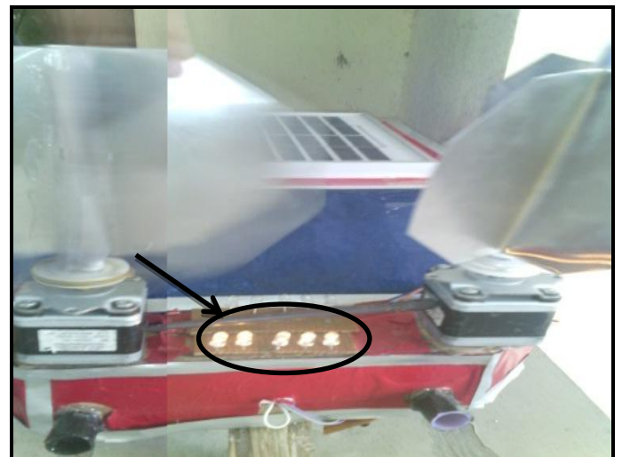
Fig -4: Glowing LEDs depicting the charging of battery when the vehicle is moving
