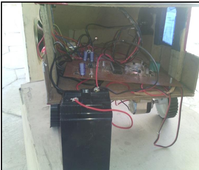
Fig -6: Circuit charging the battery using the three sources in parallel
