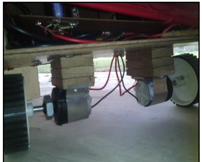
Fig -8: Motor derives the vehicle as per the microcontroller's output
