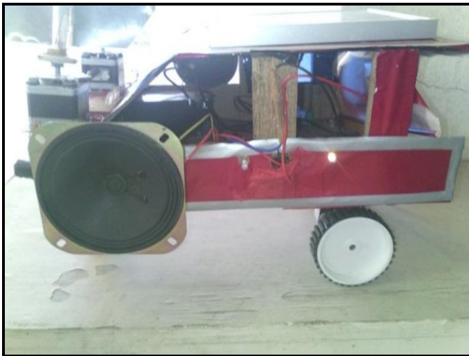
Fig -5: Piezo-electric crystal charging the battery using noise source
