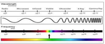
Fig -2: Electro-magnetic Spectrum
