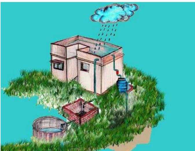
Fig- 3: Roof top rainwater harvesting.
