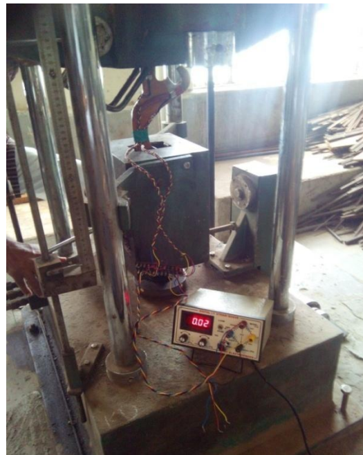
Fig -8: Experimentation at Notch 1 on ASTM A 48 C.I.
