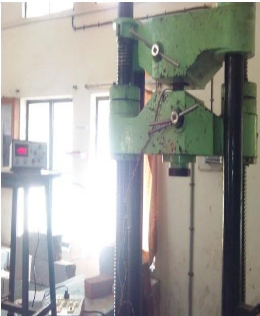
Fig -9: Experimentation at Notch 2 on ASTM A 48 C.I.
