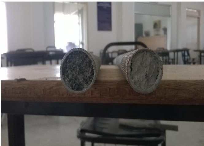
Figure.2 hollow mild steel pipe filled with rubber cement slurry
