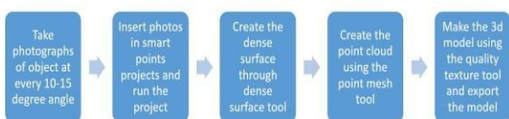
Fig - 3: Block diagram of 3D modelling
