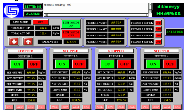
Fig- 6: HMI interface screen of LIW Feeder
