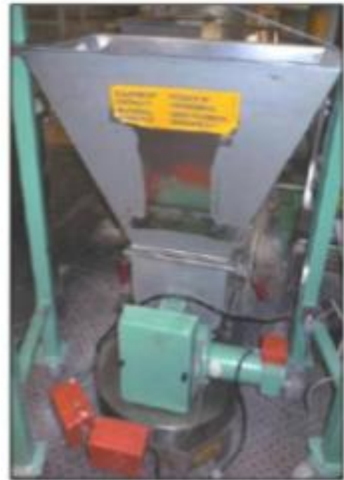
Fig- 11: LIW Feeder system installed near the plant
