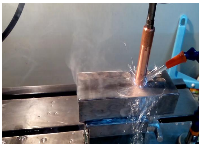
Fig -1.2.1: Flushing arrangement for discharge =2631 mm 3 /min
