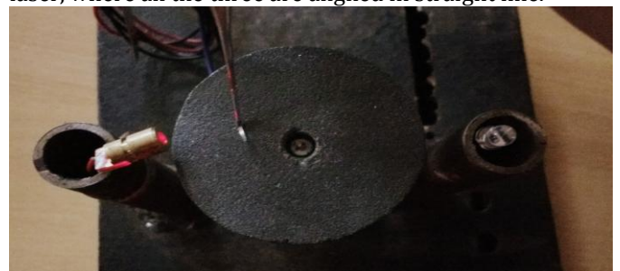
Fig-4: Laser-Phototransistor detection mechanism in proposed system
