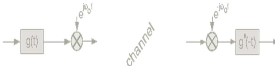
Fig-1: Basic structure of a single carrier system [4]
