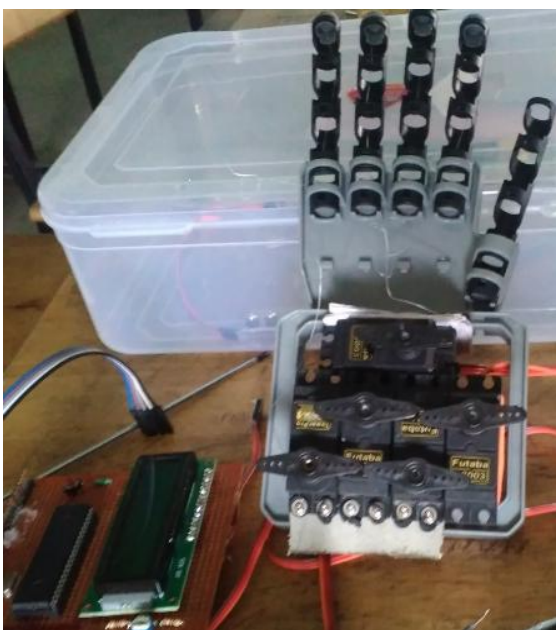
Fig-7: Set up for the Arm and servomotors
