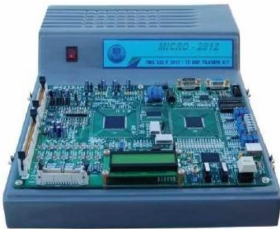
Fig- 4 DSP TMS320F2812
