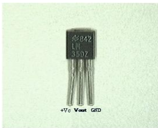
Fig-7: Temperature Sensor
