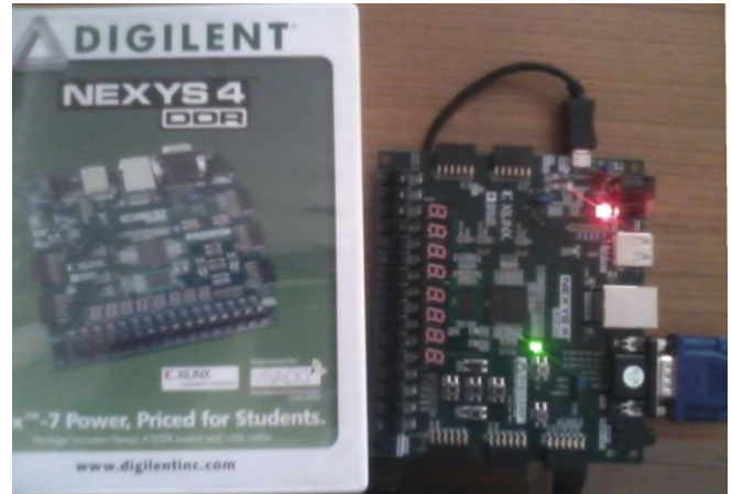
Fig 11: Artix-7 FPGA Digilent Nexys4 DDR board
