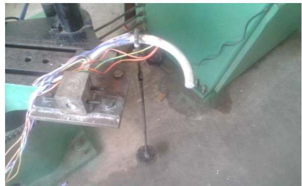
Figure 7.3- Experimental setup with weights during loading (for open angle 0 to 90deg).
