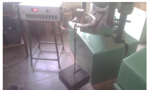
Figure 7.2- Experimental setup with weights during loading (for open angle 0 to 180deg).
