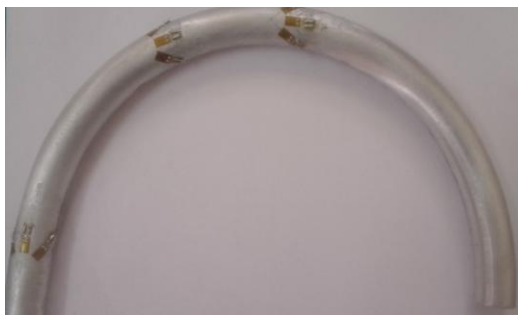
Figure 5.3 - Strain gauges mounted on specimen.
