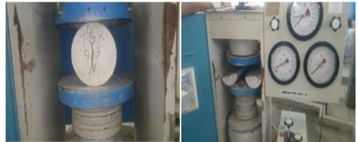
Figure -2: Testing of specimen for split tensile strength
