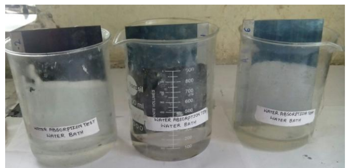
Photo 2 Water Absorption test
