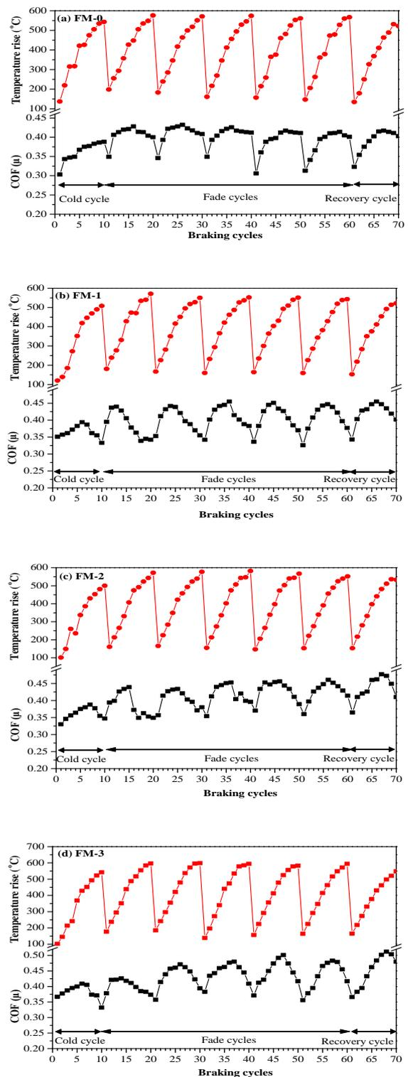
**Fig -1:** Frictional response of the brake friction materials (a) FM-0 (b) FM-1 (c) FM-2 (d) FM-3.
