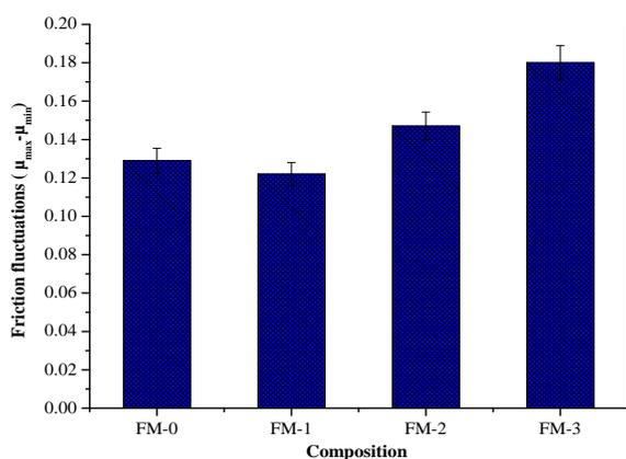
Fig -3: Frictional fluctuations of brake friction materials.
