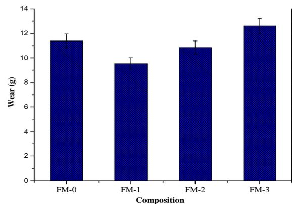
Fig -7: Wear of the brake friction materials.
