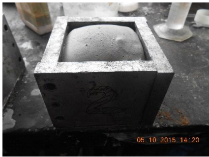
Fig.6: light weight geopolymer concrete slurry in mould at final stage
