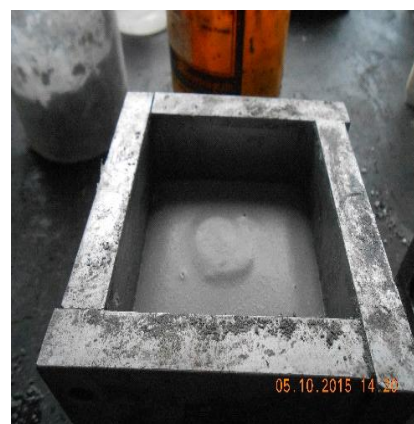
Fig.4: Light weight geopolymer concrete slurry in mould at initial stage
