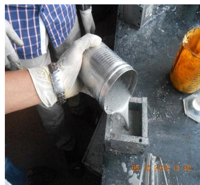
Fig.3: Casting and placing of light weight geopolymer concrete
