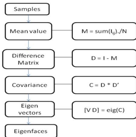
Fig - 1: PCA algorithm flow
