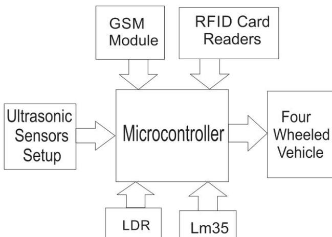
Fig -1: Block diagram of intelligent car.
