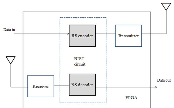
Fig-8: FPGA implementation of BIST circuit
