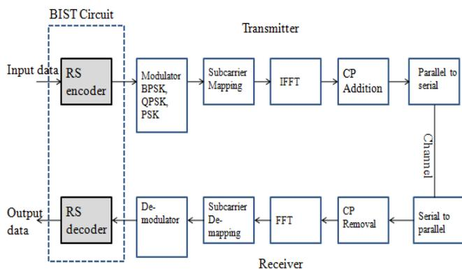
Fig-2 : Block diagram of BIST circuit in OFDM system
