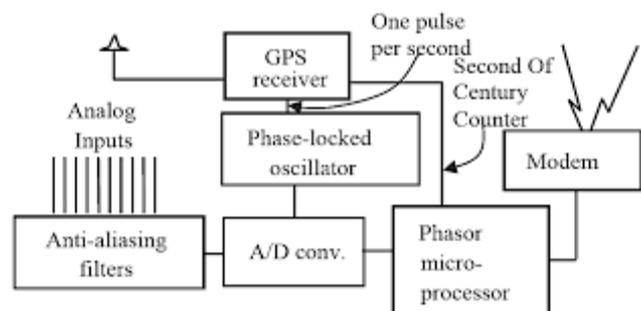
Fig. 1 – PMU Block diagram
