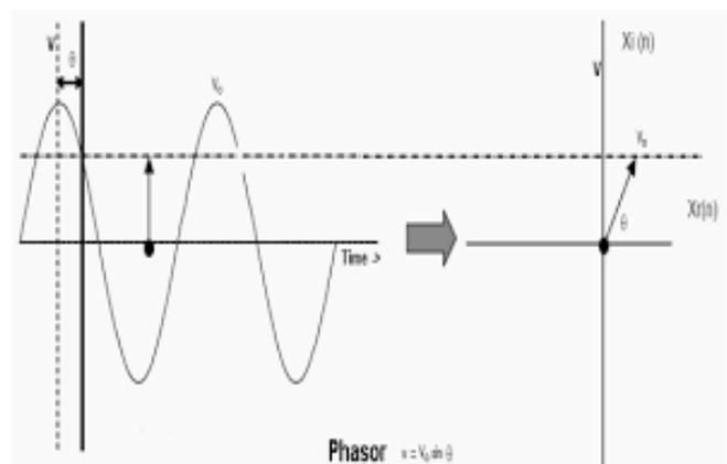
Fig. 2 Synchrophasor measurement
