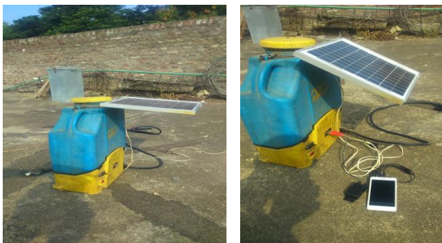
Fig.-4: Photos of Solar operated spray pump
