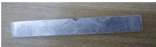
Fig. 4 Prepared Specimen for Impact toughness
