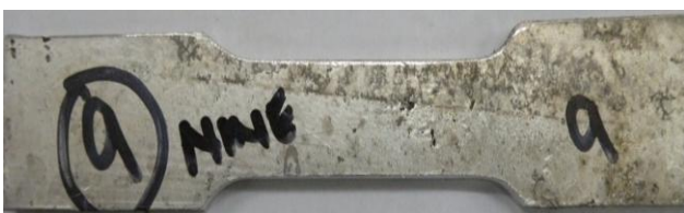
Fig.3 Prepared Specimen for Tensile Strength
