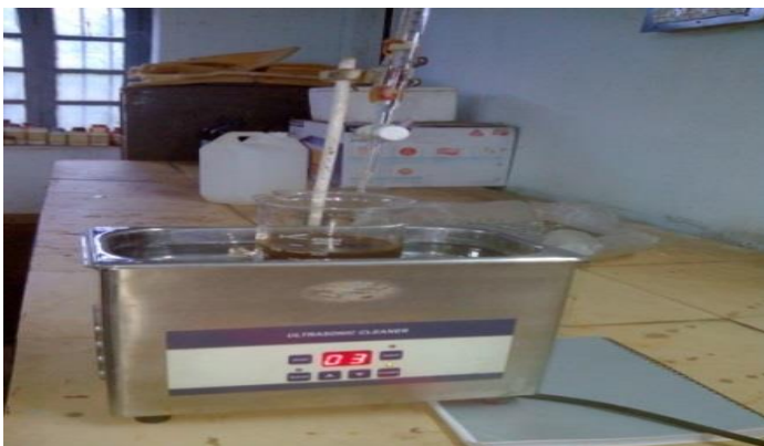
Fig-2.2 Titration of FeCl 3 and FeSO 4 using Ultra Sonication.
