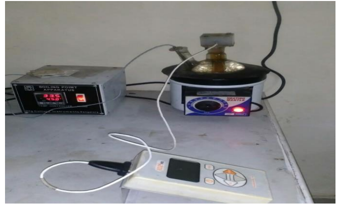
Fig-3.1 KD2 Pro instrument with water bath
