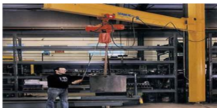
Figure 7 Mast style jib crane
