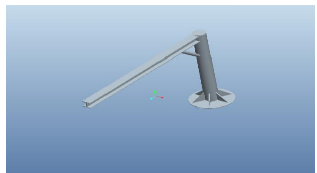
Figure 14 Reinforced jib crane assembly solid model
