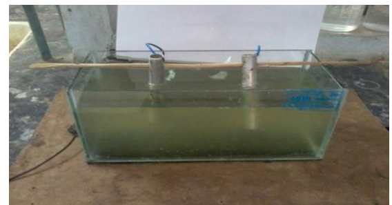
Fig 1: represents the block diagram of the electrocoagulation setup
