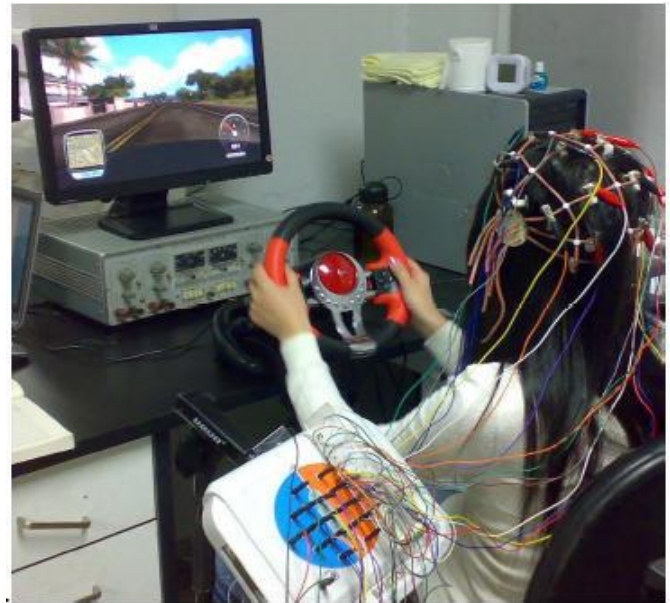
Fig -5: EEG data acquisition system[4]
