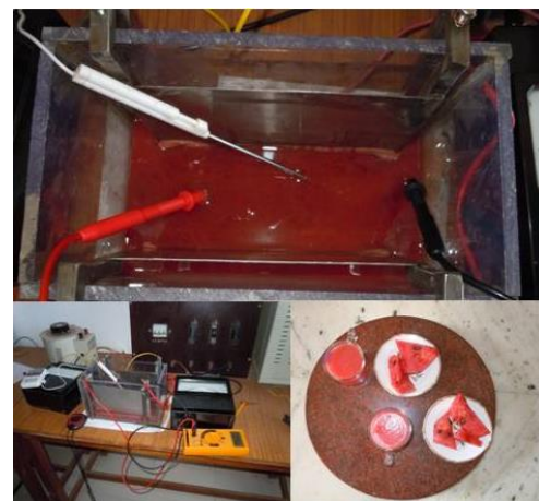
Fig. 2.Test model-OHP with Titanium electrode using lemon-water melon juice.
