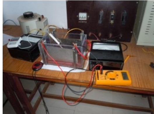
Fig 1 .Test model- OHP with Stainless steel electrode using lemon-water melon juice.
