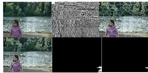
Fig-4.2 (a)Original Image (b)DWT Image (c)SLIC Segmentation (d)PSLIC Segmentation (e)Detection Result of SLIC (f)Detection Result of PSLIC
