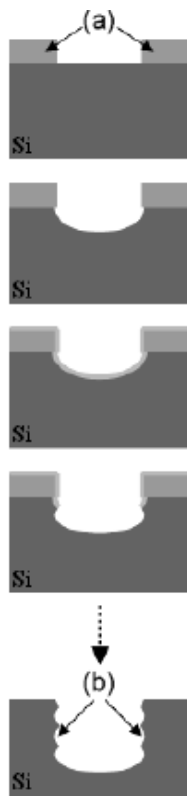
Fig -2: Example of plasma etching by the Bosch process (a – protective layer, b – vertical sidewalls)
