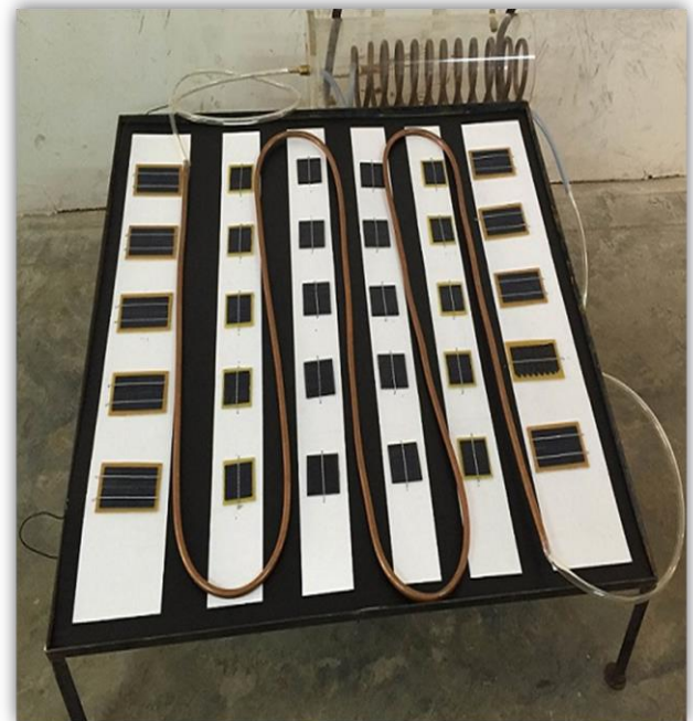
Fig -3: Portable Solar PVT power plant
