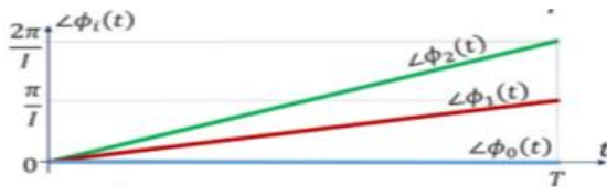
FIG.3.3 complex exponentials at multiples of a fraction of the carrier spacing (F-FFT)
