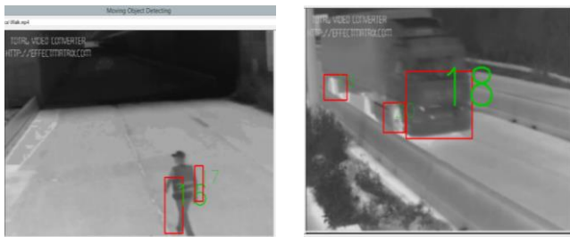
Figure 17. Processed Image for Object detection of IR Night Vision camera
