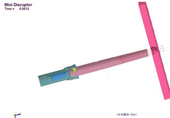
Fig.5: Water breaks the plywood in 0.001 second.
