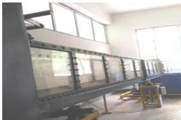
Fig-1: Rectangular channel of 6m length, 0.3m width and 0.46m depth.
