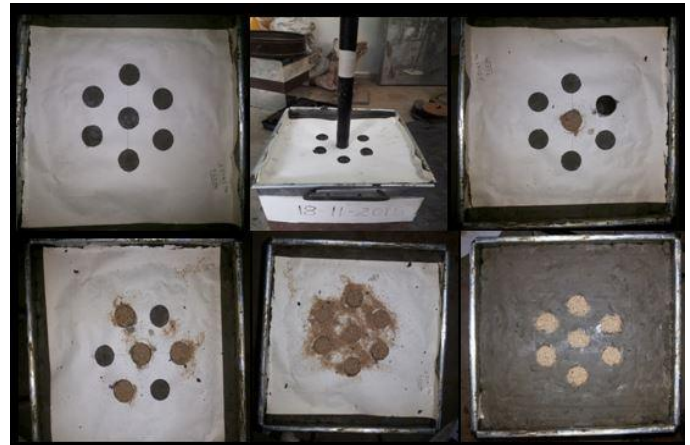
Fig.-3: Installation of Sand Pile in Prepared Clay Bed for Single Sand Pile Load Test
