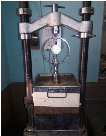
Fig-4: Experimental Setup for Single Pile Load Test
