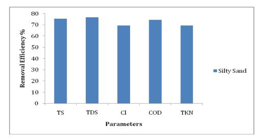
Fig 2: Removal Efficiency of all Parameters in Silty Sand Soil with Adsorbents at 50% Height
