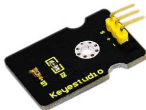
Fig. 5. TEMT6000 Light Intensity Monitoring sensor.
