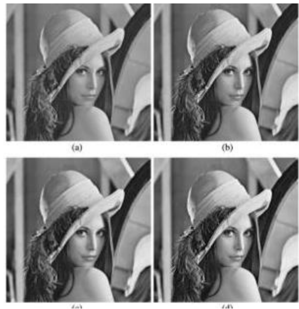
Fig. 3. The original and contrast-enhanced images of "Lena" by splitting 10, 15 and 20 pairs of histogram peaks in the proposed algorithm. (a) Original image of "Lena". (b) 10 pairs: 0.185 bpp, 29.10 dB. (c) 15 pairs: 0.268 bpp, 25.97 dB. (d) 20 pairs: 0.345 bpp, 24.91 dB.
