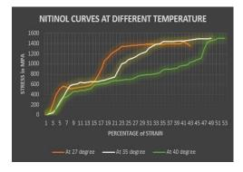
Fig 7: Combined Strain Curve for Nitinol at all Working Temperature
