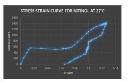
Fig 4: Strain Curve for Nitinol at 27  $^\circ\text{C}$
