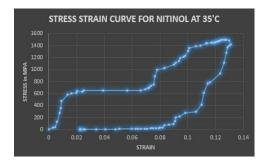
Fig 5: Strain Curve for Nitinol at 35 °C
