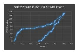
Fig 6: Strain Curve for Nitinol at 40 °C
