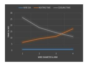
Fig 9: Plot of Wire Diameter V/S Time
