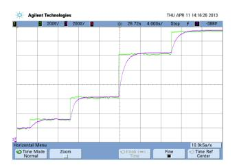
Figure 9 Dynamic speed waveform of PI-ILC-SVPWM
