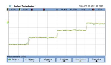
Figure 7 Dynamic speed waveform of PI-SVPWM
