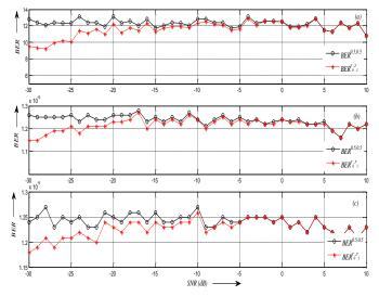
**Fig -5:** *BER* vs. *SNR* curve corresponding to sound samples, for a)  $N_w = 1000$  b)  $N_w = 5000$  c)  $N_w = 10,000$
