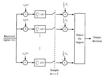
Fig -2: Block diagram of optimum receiver [6]
