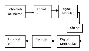
Fig -1: Block Diagram of Digital Communication
