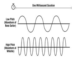
**Fig -4:** Relationship between pitch and frequency of sound [8]
