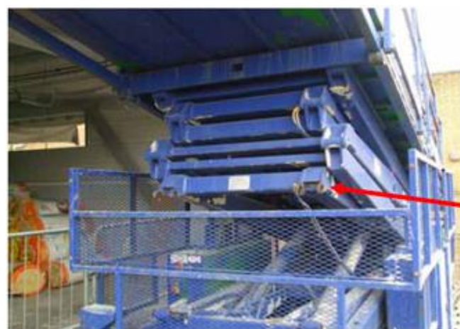
Fig:(5): Failure of Hydraulic Scissor lift due to maximum deformations
