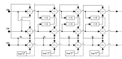
Fig -1: Unfolded CORDIC structure
