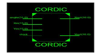
Fig -1: RTL Schematic of CORDIC Processor
