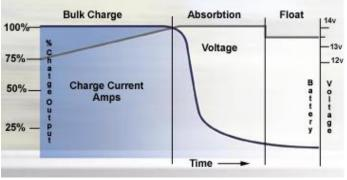
Fig-2: Three different charging modes of Battery
