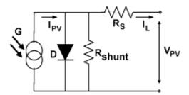
Fig-3: equivalent circuit of a PV cell
