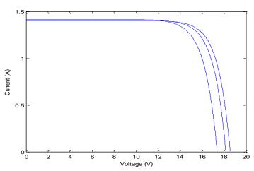
Fig-7: The effect of temperature on the V-I of PV Panels
