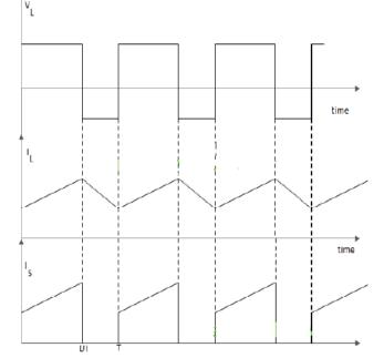
Fig-11: Waveform of Boost converter
