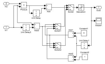
Fig-15: SIMULINK model of P&O Algorithm
