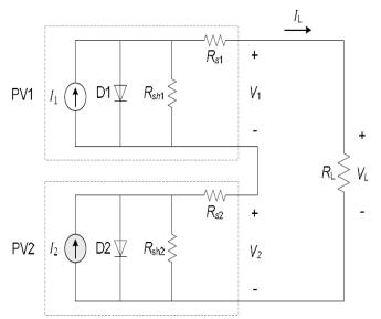
Fig-12: Two PV modules connected in series under shaded
