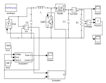
Fig-14: SIMULINK model of boost converter with P&O MPPT
