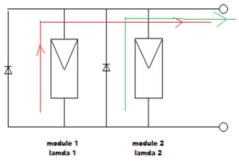
Fig-20: Two parallel connected panels with bypass diodes
