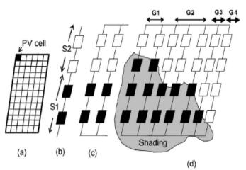
Fig-4: PV array,(a) PV module (b) Series-assembly with two series-connected subassemblies S1 and S2 (c) Group. (d) PV array with groups G1 to G4.
