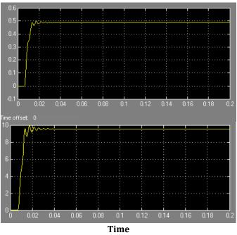
Fig-16: output I & V of boost converter with respect to Time
