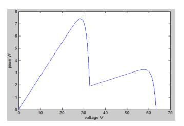
Fig-19:chara. of two series connected panel under shaded
