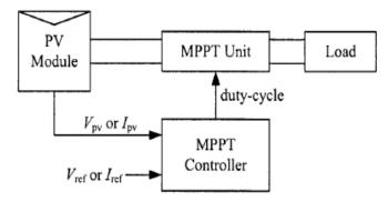
Fig-5: Typical MPPT control system
