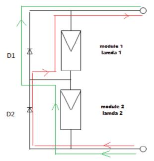
Fig-18: Two series connected modules with bypass diode
