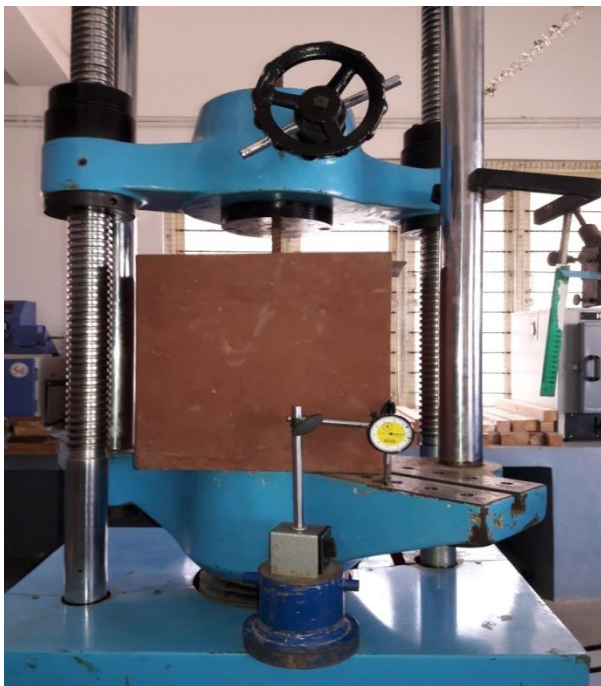
Fig 1.0 Experimental setup with a square tank and dial gauge
