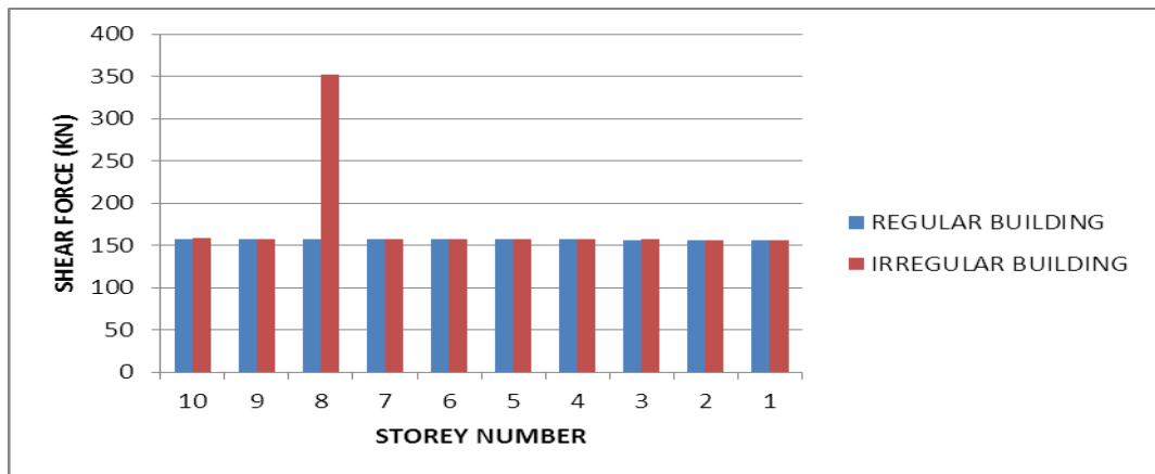
Figure 4.8 Storey wise maximum shear force in beams
