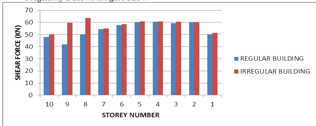
Figure 4.11 Storey wise maximum shear force in columns
